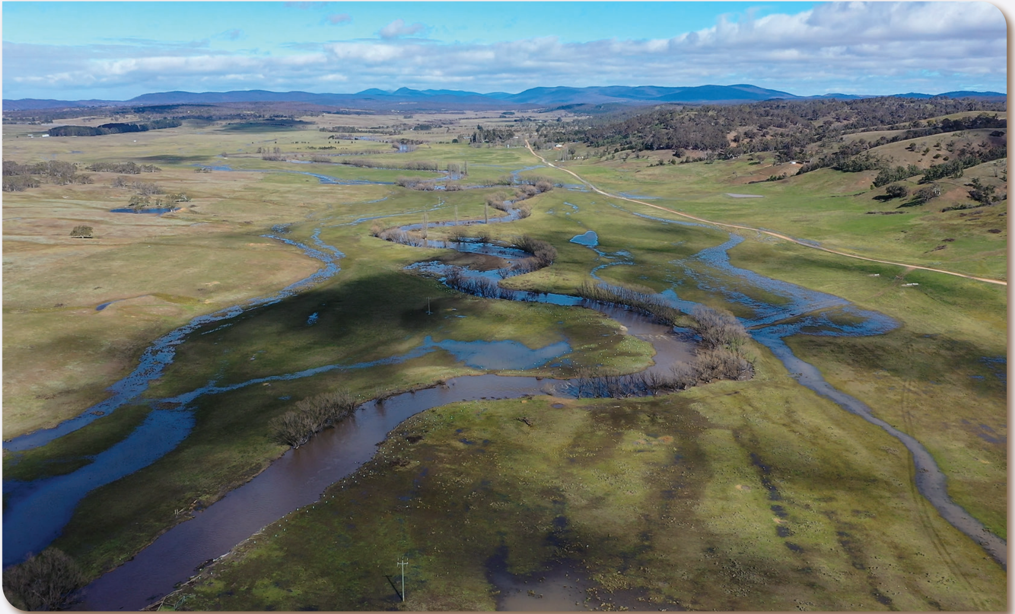
Figure 95: Mulloon Creek, August 2020, with floodwaters receding. Multiple in-stream structures attenuated the high flows, and caused water to safely overbank and spill across the floodplain. As a result, water reached secondary and tertiary channels, extending the hydrating footprint of the flood, and tonnes of nutrient-rich sediment were deposited across the floodplain.
