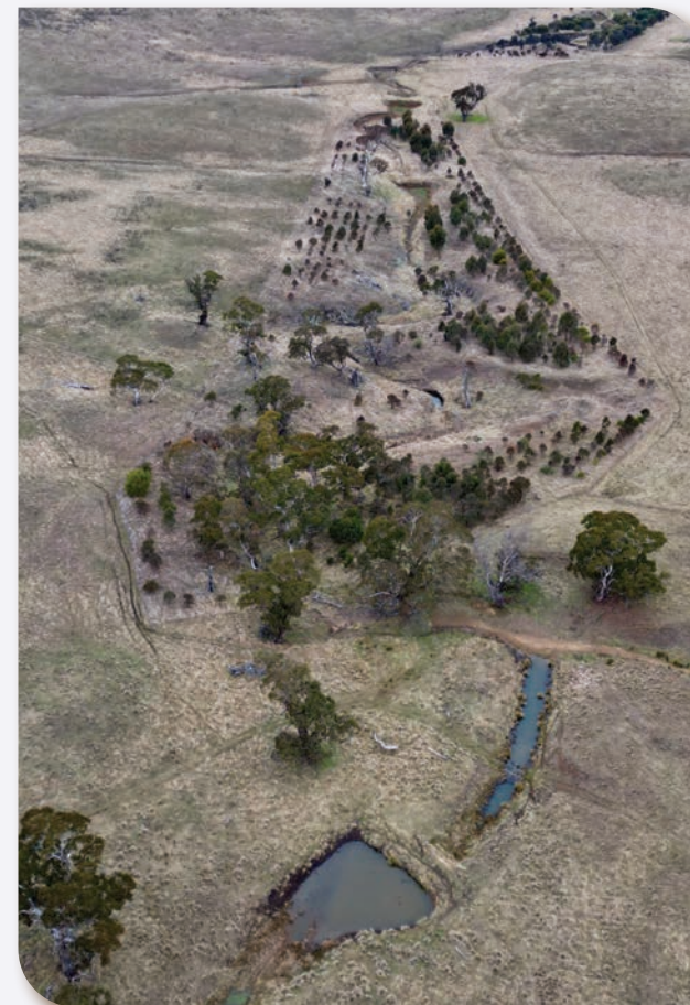
Figure 29: A formerly incised stream with active erosion that has been repaired with natural infrastructure and improved land management in the Monaro region. The scar of the incision is still clearly visible, however the site is regenerating due to plantings, a grazing regime that maintains 100% groundcover, and a series of ponds. Photo by Charlie Maslin.
